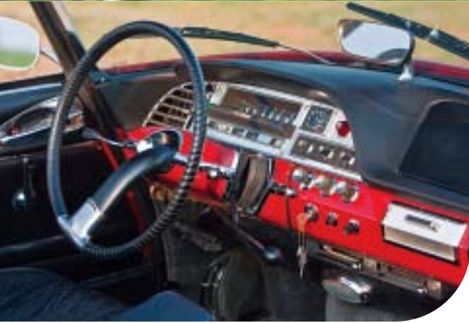
» » » » » Top: Passing through a Virginia winery. Above, from left: The DS's dash is a hodgepodge of unlabeled switches and beautifully finished stainless steel (note the suspension-height lever in the footwell); the vent controls are almost aeronautical; clutch, brake, throttle. Below: Greg Long in his Charlottesville garage.
