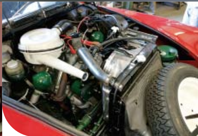
» » » » » Clockwise from top: Leaving Seattle; the green globes on each side of the engine bay are the hydraulic spheres for the front suspension; a gutted DS sedan behind Chris M.'s Seattle shop; the Citroën stares at the moon in eastern Washington; the DS's rubber-mushroom brake "pedal" assembly, removed and sectioned for display.
