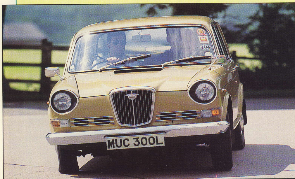
Wolseley Six offered six-cylinder refinement allied to the spacious interior of the BMC 1800 body with its wide track. Hydrolastic suspension and transverse six-cylinder OHC engine driving the front wheels were novel in its class
