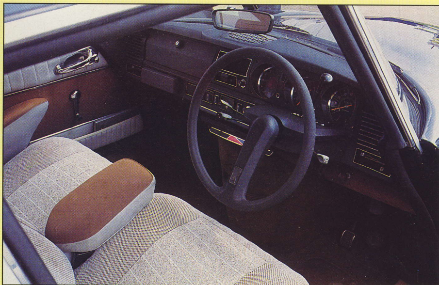
Citroën DS23 featured highly individual styling and an advanced technical specification. Interior combines Pallas luxury trim with Citroën idiosyncrasies of rubber-button brake pedal and single-spoke steering wheel
